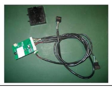
10.5 Disconnect the screw fastening FRONT IO bracket to the case, disconnect the button cable and the screw , then rotate bracket finger outward, and pull out the FRONT IO
